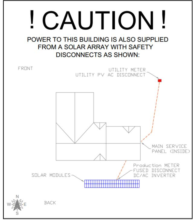
Figure 11. Metering Profile Elevation Drawing
