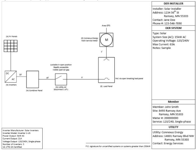
Figure 7. Example of Typical One-line Diagram of Solar DER
